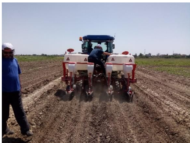
Figure 1. Seeder applying liquid fertilizer to the soil
