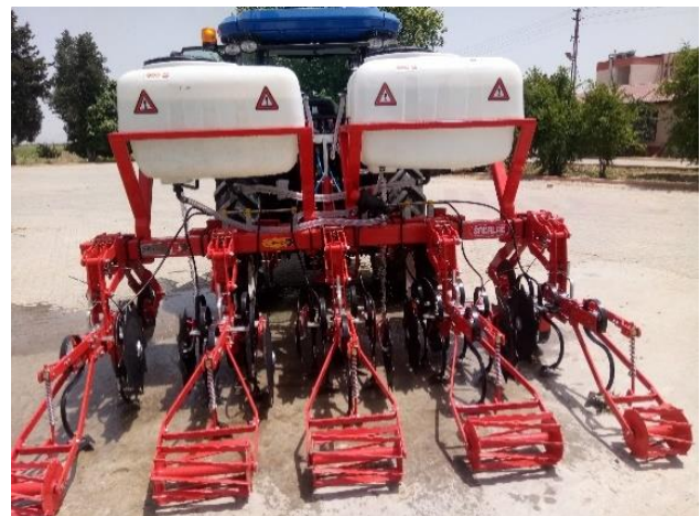
Figure 2. Machine applying both hoe and liquid fertilizer
