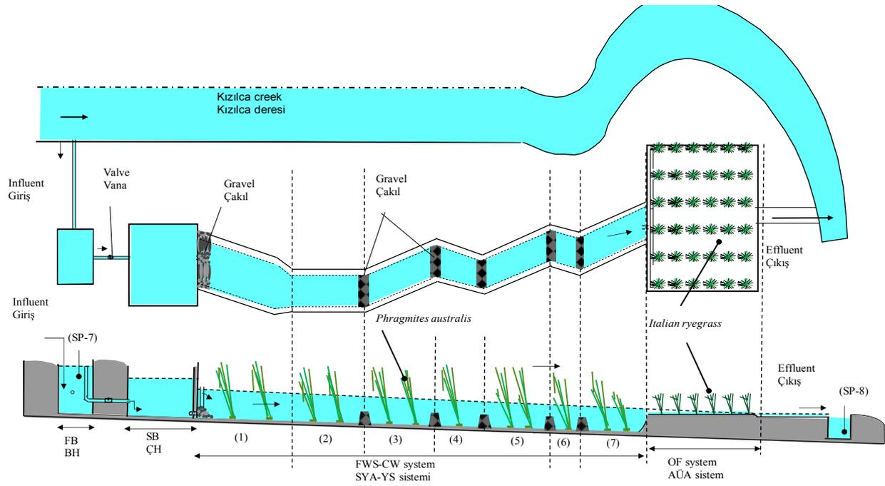
Figure 1. Schematic diagram of the hybrid NWT (SP-7 and SP-8 are sampling locations) system.
